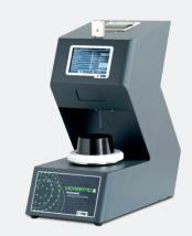
The setting time determination of cement/mortar/gypsum is one of the most important parameter for the quality inspection and verification.
