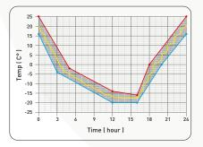
The user can preset the time and target temperature of each ramp and the number of each set by using the control unit.
