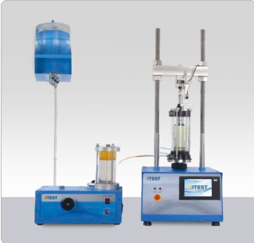
UU Only Triaxial Test Configuration
