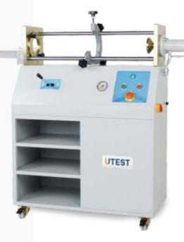
The Hand Operated Hydraulic Extruder is supplied complete with;
