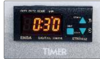
Sand Equivalent Shaker Timer
